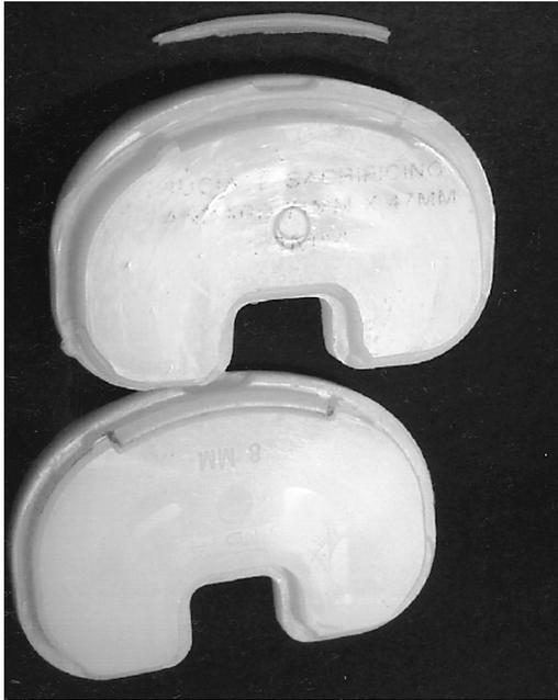
**Fig 4.** Backside wear and fatigue failure of anterior locking tab on a modular polyethylene insert are shown.
